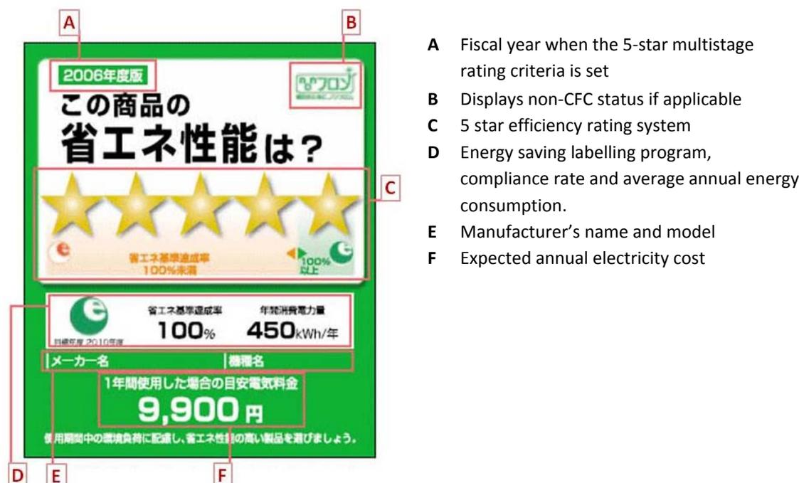
The label on an air conditioner on the Japanese market (Figure 19) also includes an estimate of the annual volume of kilowatt hours (kWh) used for heating and cooling. The inclusion of data on
