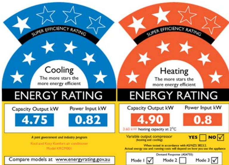
It is mandatory for air conditioners sold in Australia to include an energy efficiency label in the format illustrated in Figure 16.
